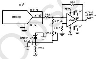
FIGURE 5. Bipolar Operation
