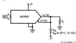
FIGURE 4. Improving Negative Slew Rate
