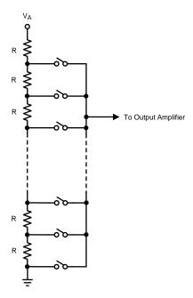
Figure 37. DAC Resistor String
