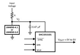
Figure 44. The LM4050 as a power supply
