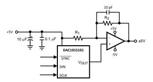
Figure 47. Bipolar Operation
