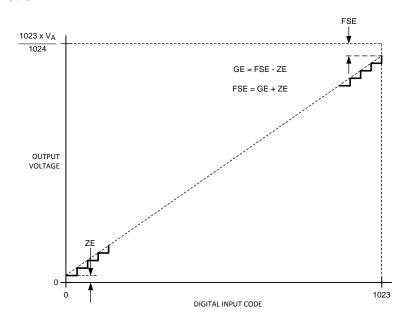
Figure 3. Input / Output Transfer Characteristic
