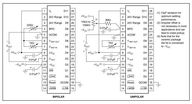
FIGURE 5. Power Supply, Gain, and Offset Connections.
