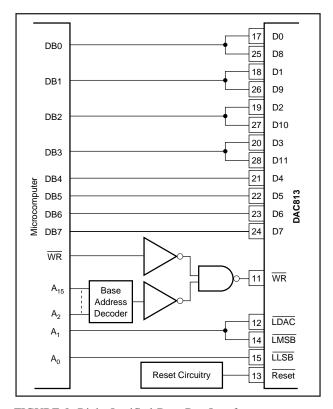
FIGURE 8. Right-Justified Data Bus Interface.
