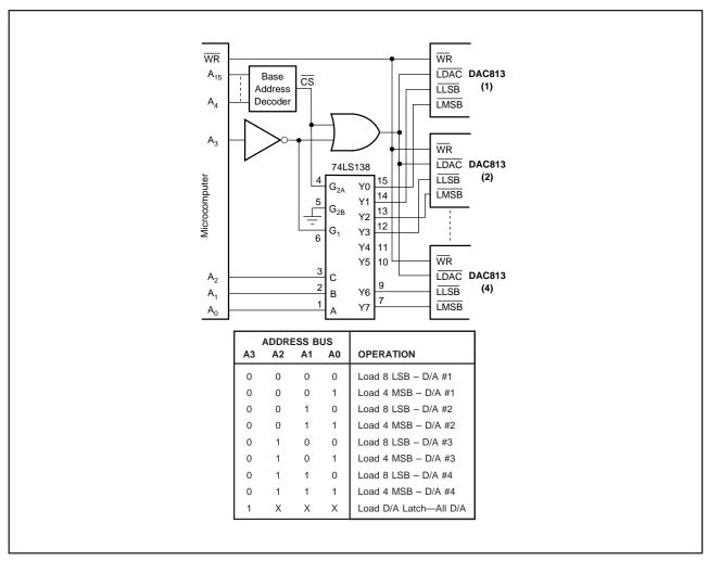
FIGURE 9. Interfacing Multiple DAC813s to an 8-Bit Bus.
