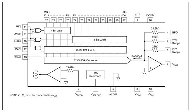
FIGURE 1. DAC813 Block Diagram.
