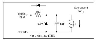
FIGURE 2. Equivalent Input Circuit for Digital Inputs.
