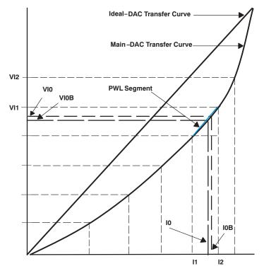
Figure 21. The Geometry Behind the PWL Calibration
