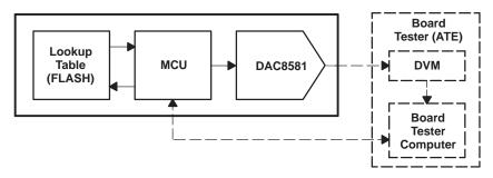
Figure 20. Production Test Setup for a DAC8581 Board With Calibration
