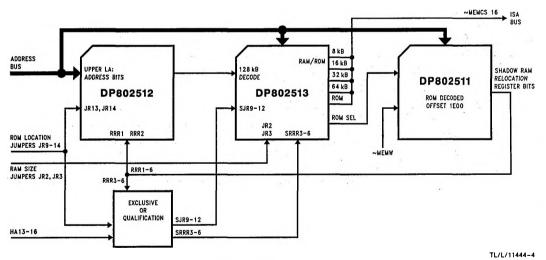
FIGURE 2. MEMCS\_\_16 Logic
