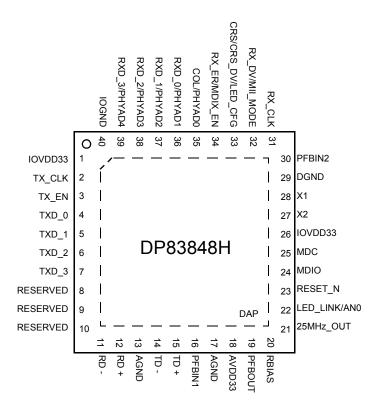
Note: Die Attached Pad (DAP) provides thermal dissipation, connection to GND plane recommended.
