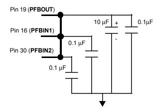
Figure 13. Power Feeback Connection
