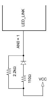
Figure 3. ANO Strapping and LED Loading Example
