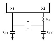
Figure 12. Crystal Oscillator Circuit
