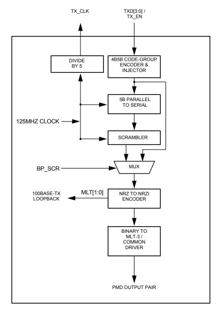
Figure 6. 100BASE-TX Transmit Block Diagram
