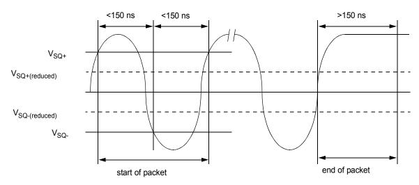
Figure 10. 10BASE-T Twisted Pair Smart Squelch Operation
