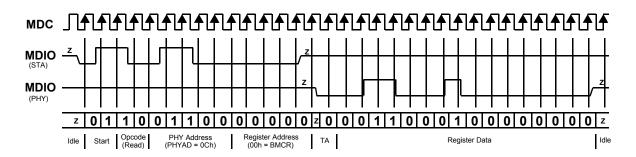
Figure 4. Typical MDC/MDIO Read Operation
