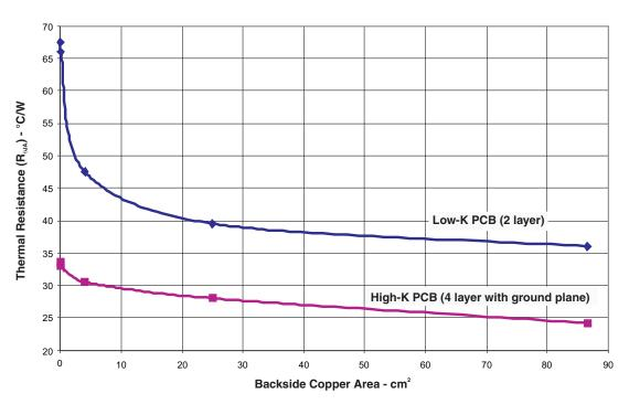
Figure 3. Thermal Resistance vs. Copper Plane Area
