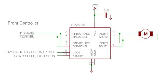
Figure 1. Parallel Mode Connections
