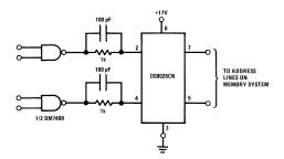
Figure 7. DC Coupled RAM Memory Address or Precharge Driver (Positive Supply Only)
