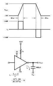
Figure 9. Clock Waveforms (Voltage and Current)
