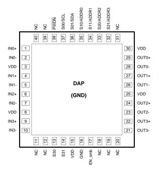
Figure 1. WQFN Package See Package Number RTA0040A
