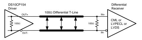
Figure 5. Typical DS10CP154A Output DC-Coupled Interface to an LVDS, CML or LVPECL Receiver
