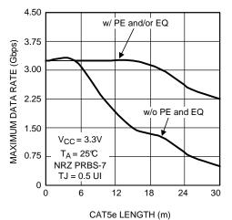
Figure 15. Maximum Data Rate as a Function of CAT5e (Belden 1700A) Length
