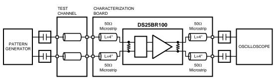
Figure 6. Equalization Performance Test Circuit
