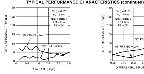
Figure 18. Total Jitter as a Function of Data Rate
