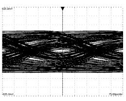
Figure 13. A 2.5 Gbps NRZ PRBS-7 After 60" Differential FR-4 Stripline V:125 mV / DIV, H:75 ps / DIV
