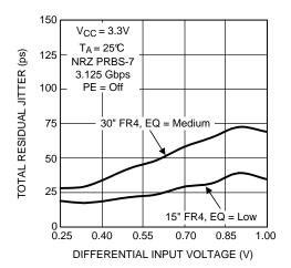
Figure 22. Total Jitter as a Function of Input Amplitude
