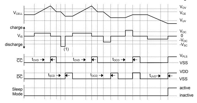
(1) To allow the device to react quickly to short circuits, detection is actually done on the SNS pin rather than on the filtered IS1 and IS2 pins. The actual short circuit detect condition is  $V_{\text{SNS}} > V_{\text{SC}}$ .
