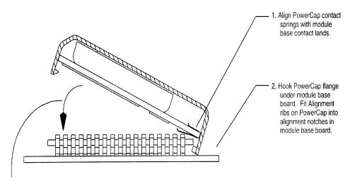
3. Pushdown and forward with screwdriver while inserting the PowerCap. This action will "open" the attachment feature.
