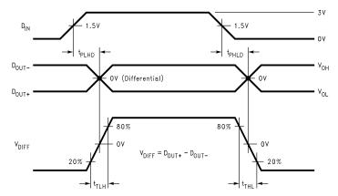
Figure 5. Driver Propagation Delay and Transition Time Waveforms
