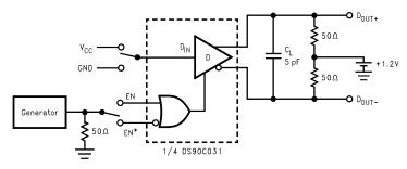
Figure 6. Driver TRI-STATE Delay Test Circuit
