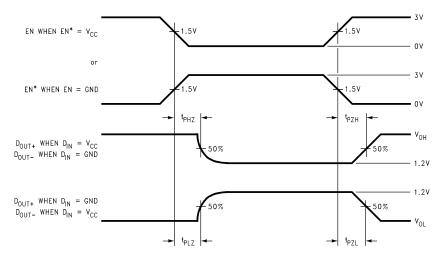
Figure 7. Driver TRI-STATE Delay Waveform
