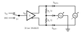
Figure 3. Driver V<sub>OD</sub> and V<sub>OS</sub> Test Circuit
