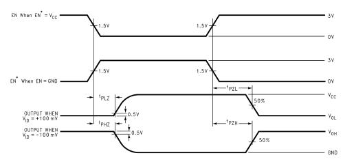
Figure 6. Receiver TRI-STATE Delay Waveforms
