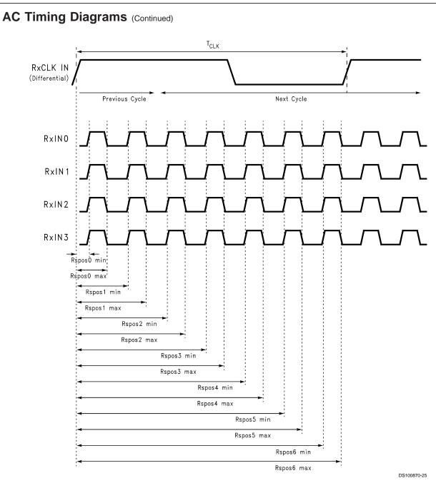
FIGURE 11. DS90CF384A (Receiver) LVDS Input Strobe Position
