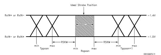
C—Setup and Hold Time (Internal data sampling window) defined by Rspos (receiver input strobe position) min and max Tppos—Transmitter output pulse position (min and max)
