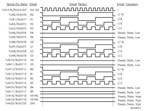
FIGURE 3. "16 Grayscale" Test Pattern (DS90CF364A)(Notes 5, 6, 7, 8)
