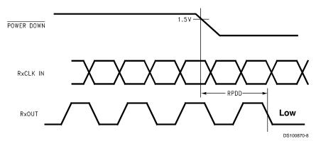
FIGURE 10. DS90CF384A/DS90CF364A (Receiver) Power Down Delay
