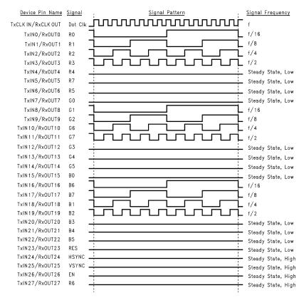
The worst case test pattern produces a maximum toggling of digital circuits, LVDS I/O and CMOS/TTL I/O.
