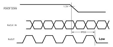
Figure 9. Receiver Power Down Delay
