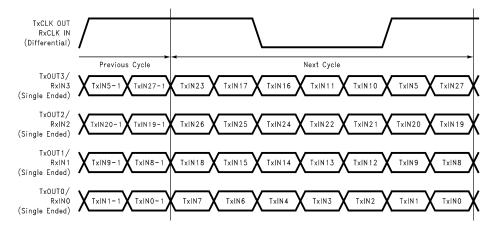
Figure 8. 28 Parallel TTL Data Inputs/Outputs Mapped to LVDS Bits (TxlNn / RxOUTn)
