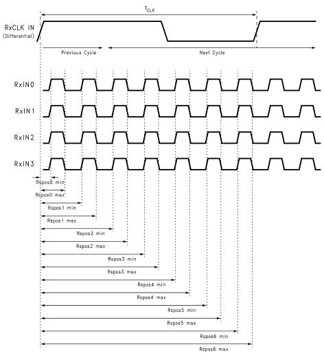
Figure 10. Receiver LVDS Input Strobe Position
