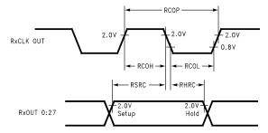
Figure 5. Receiver Output Setup/Hold and High/Low Times
