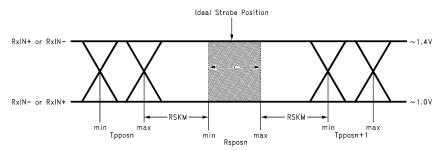
C—Setup and Hold Time (Internal data sampling window) defined by Rspos (receiver input strobe position) min and max
