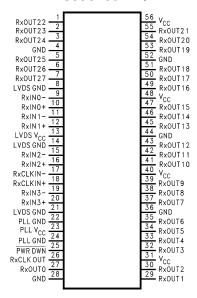
Figure 12. 56-Lead TSSOP (DGG Package)
