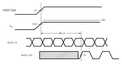
Figure 7. Receiver Phase Lock Loop Set Time
