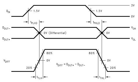
Figure 4. Driver Propagation Delay and Transition Time Waveforms
