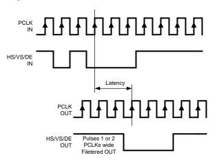
Figure 12. Video Control Signal Filter Waveform
