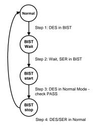
Figure 18. BIST Mode Flow Diagram
