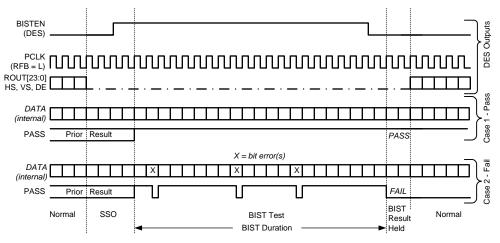
Figure 19. BIST Waveforms
