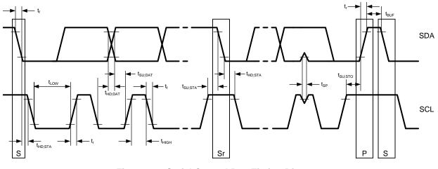
Figure 10. Serial Control Bus Timing Diagram
