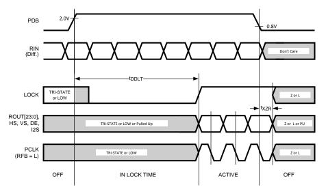
Figure 6. PLL Lock Times and PDB TRI-STATE Delay
