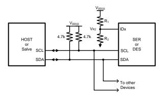
Figure 20. Serial Control Bus Connection
