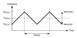
Figure 13. SSCG Waveform
