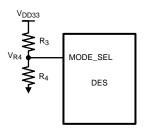
Figure 14. MODE\_SEL Connection Diagram
