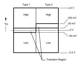
Figure 2. M-LVDS Receiver Input Thresholds
