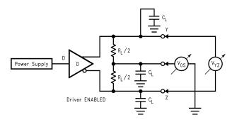
Figure 3. Differential Driver Test Circuit
