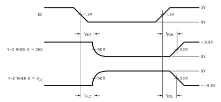
Figure 11. Driver TRI-STATE Delay Waveforms
