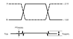
Figure 4. Differential Driver Waveforms
