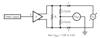
Figure 5. Differential Driver Full Load Test Circuit
