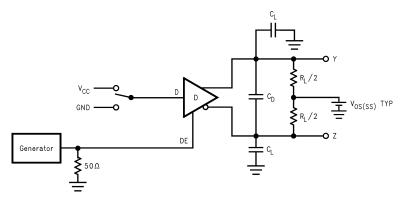
Figure 10. Driver TRI-STATE Delay Test Circuit
