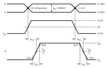
Figure 14. Type 2 Receiver Propagation Delay and Transition Time Waveforms
