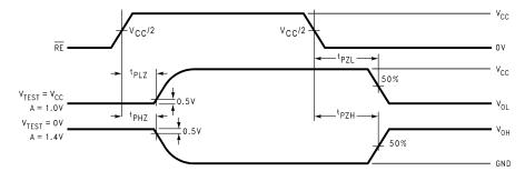
Figure 16. Receiver TRI-STATE Delay Waveforms
