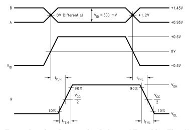
Figure 13. Type 1 Receiver Propagation Delay and Transition Time Waveforms
