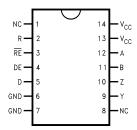
Figure 1. Connection Diagram
