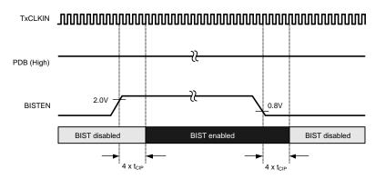
Figure 18. BIST Test Enabled/Disabled
