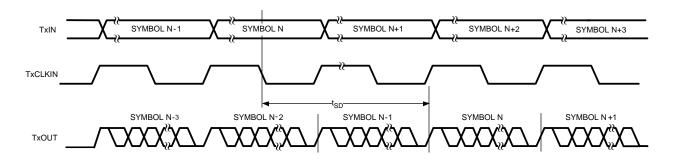
Figure 8. Serializer Propagation Delay
