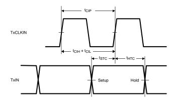
Figure 7. Serializer Setup/Hold and High/Low Times
