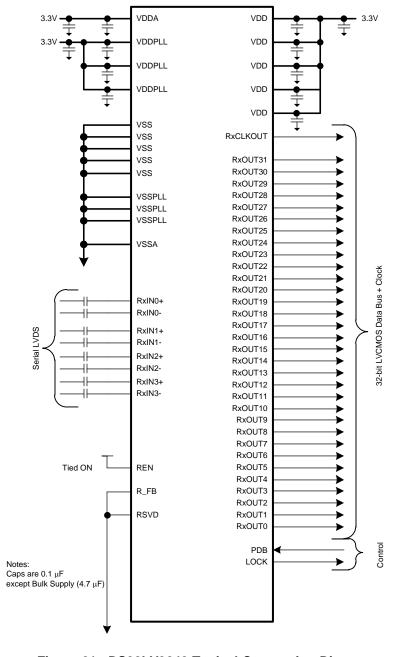
Figure 21. DS92LV3242 Typical Connection Diagram
