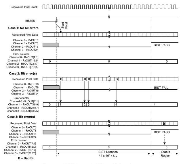
Figure 19. BIST Diagram for Different Bit Error Cases
