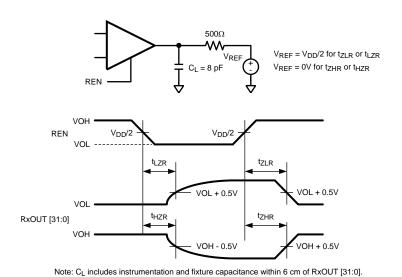
Figure 14. Deserializer TRI\_STATE Test Circuit and Timing
