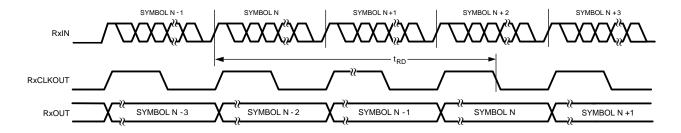
Figure 12. Deserializer Propagation Delay
