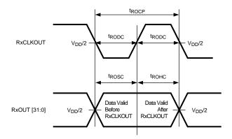
Figure 11. Deserializer Setup and Hold times
