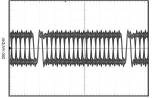
Figure 22. Serial Output Quad Mode, 85 MHz, VSEL = H, No Pre-Emphasis
