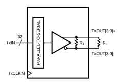
Figure 16. Serializer V<sub>OD</sub> Test Circuit Diagram
