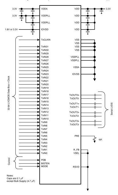
Figure 20. DS92LV3241 Typical Connection Diagram
