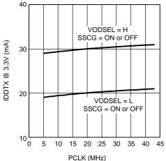
Figure 14. Typical IDDTX Current (3.3V Supply) as a Function of PCLK
