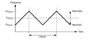
Figure 17. SSCG Waveform
