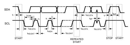
Figure 11. Serial Control Bus Timing Diagram
