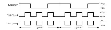
Figure 2. Checkerboard Data Pattern
