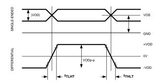
Figure 7. FPD-Link (LVDS) Single-ended and Differential Waveforms
