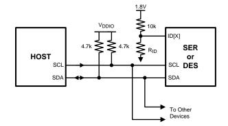
Figure 20. Serial Control Bus Connection
