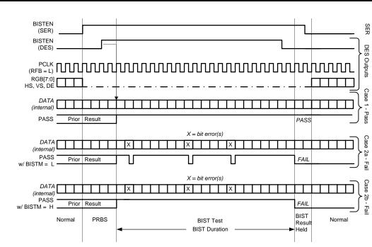
Figure 19. BIST Waveforms
