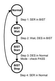
Figure 18. BIST Mode Flow Diagram
