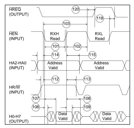
Host Figure 3. Host Read Cycle (Non-DMA Mode)
