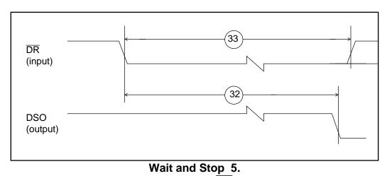
Recovery from WAIT/STOP State Using DR Pin— Asynchronous Timing
