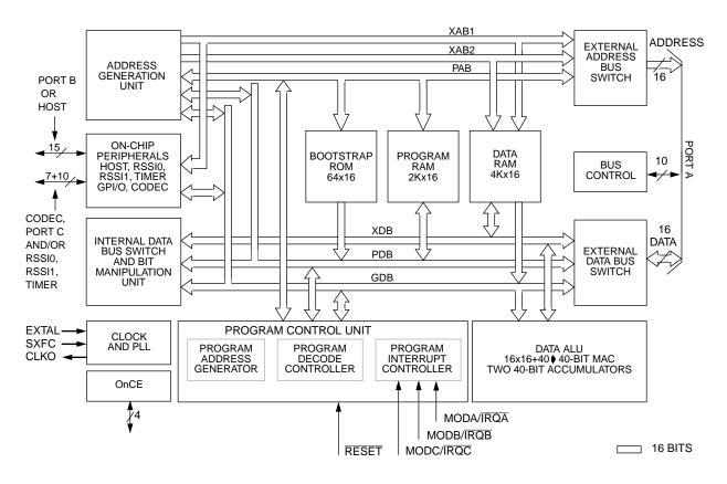
Figure 1 DSP56166 Block Diagram
