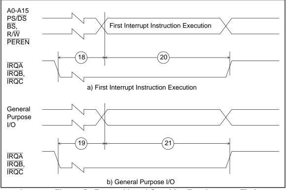
Interrupt Figure 5. External Level-Sensitive Fast Interrupt Timing
