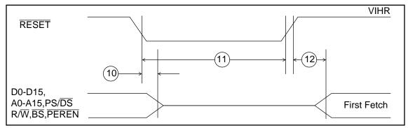
Interrupt Figure 1. Asynchronous Reset Timing
