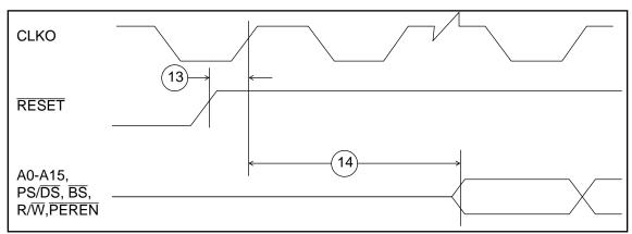
Interrupt Figure 2. Synchronous Reset Timing
