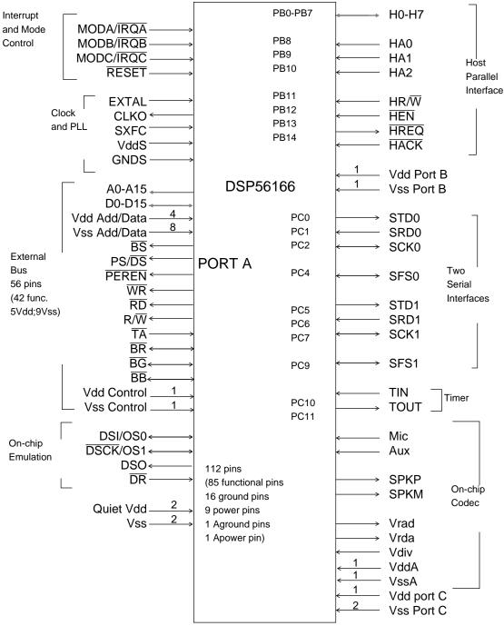
Figure 3 DSP56166 Pinout
