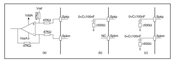
Analog I/O Figure 2. Single-ended Output Configurations
