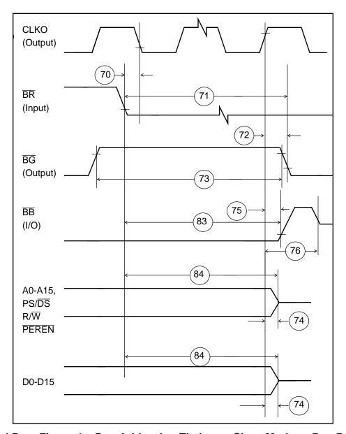
External Bus Figure 4. Bus Arbitration Timing — Slave Mode — Bus Release.
