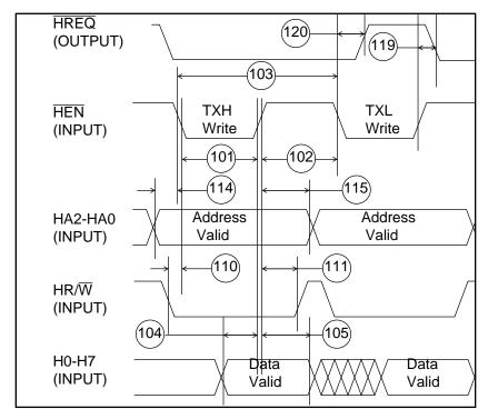
Host Figure 4. Host Write Cycle (Non-DMA Mode)
