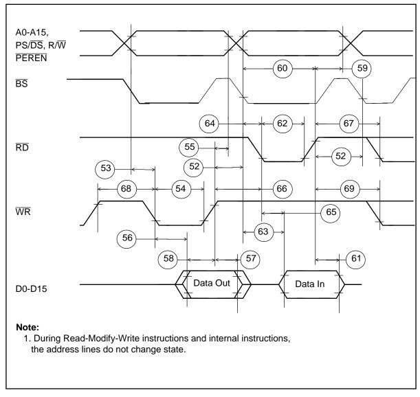
External Bus Figure 3. External Bus Asynchronous Timing
