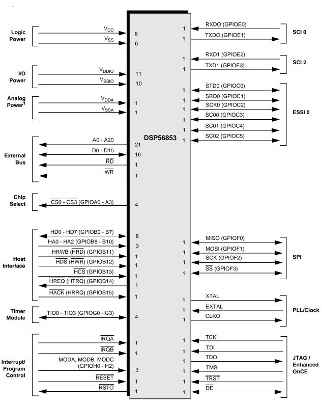
Figure 2. DSP56853 Signals Identified by Functional Group<sup>2</sup>
