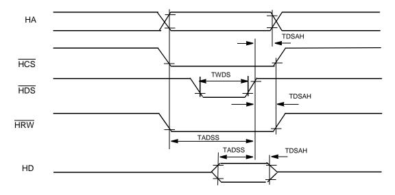
Figure 22. Single Strobe Write Mode
