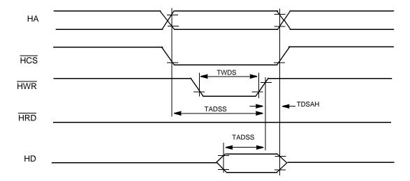
Figure 23. Dual Strobe Write Mode
