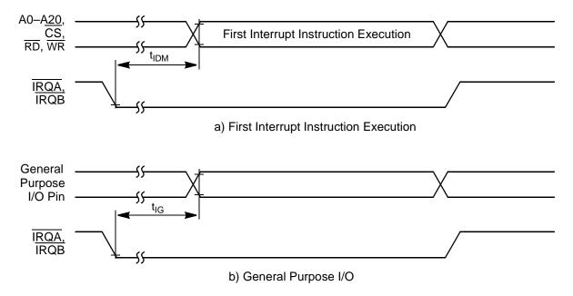
Figure 14. External Level-Sensitive Interrupt Timing
