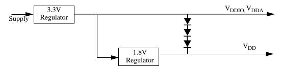
Figure 4. Example Circuit to Control Supply Sequencing
