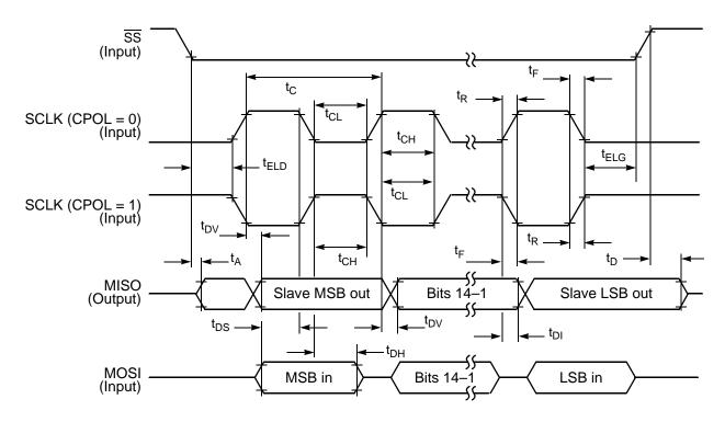
Figure 27. SPI Slave Timing (CPHA = 1)
