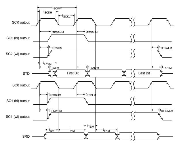
Figure 29. Master Mode Timing Diagram
