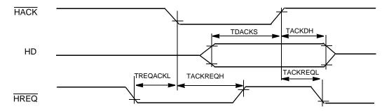
Figure 21. Host-to-DSP DMA Write Mode
