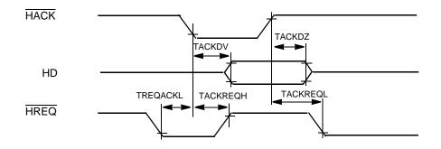
Figure 18. DSP-to-Host DMA Read Mode
