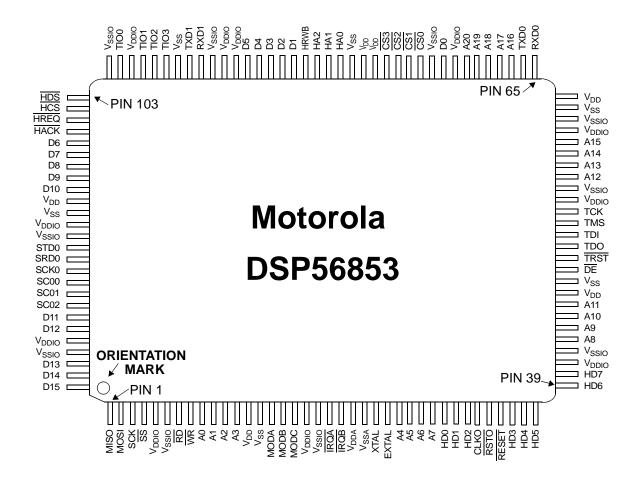
Figure 38. Top View, DSP56853 128-pin LQFP Package
