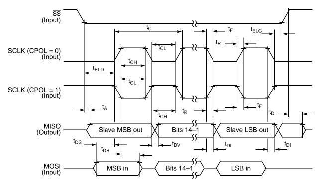
Figure 26. SPI Slave Timing (CPHA = 0)
