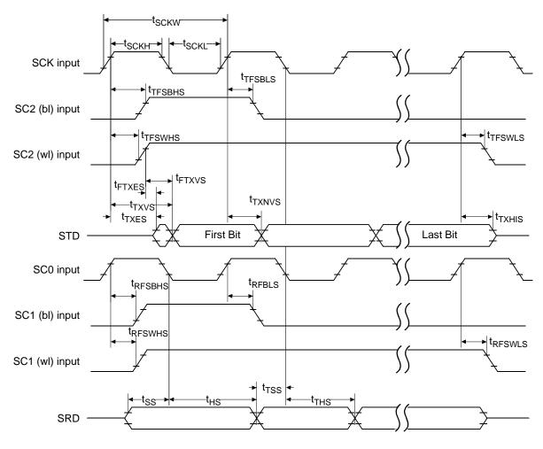
Figure 30. Slave Mode Clock Timing
