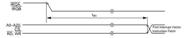
Figure 15. Interrupt from Wait State Timing
