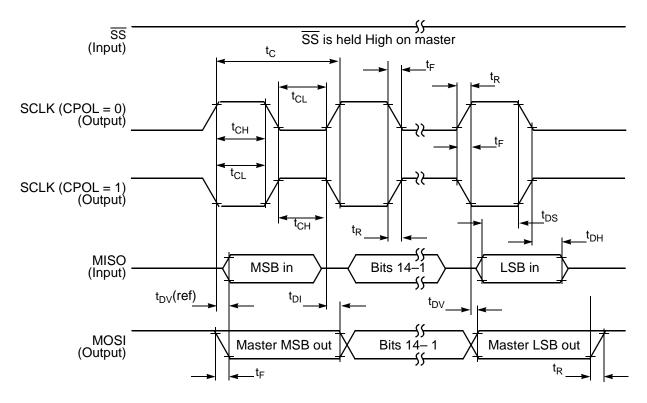
Figure 25. SPI Master Timing (CPHA = 1)
