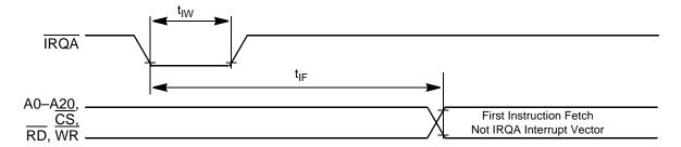
Figure 16. Recovery from Stop State Using Asynchronous Interrupt Timing
