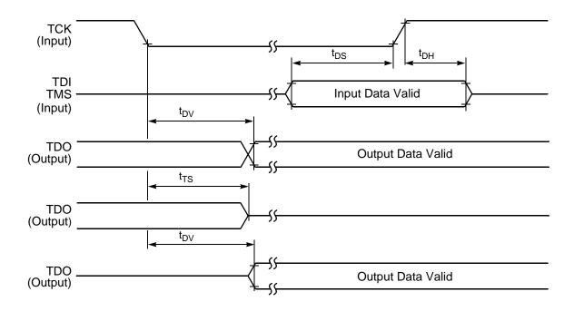
Figure 32. Test Access Port Timing Diagram
