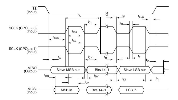
Figure 24. SPI Slave Timing (CPHA = 0)
