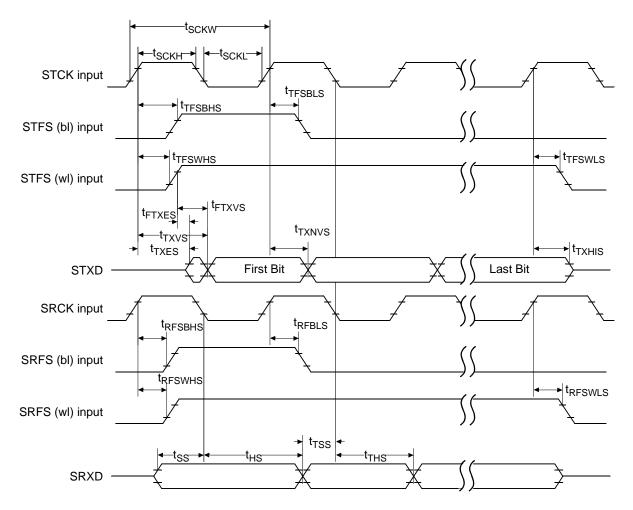
Figure 27. Slave Mode Clock Timing
