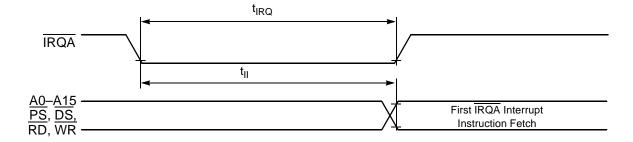
Figure 21. Recovery from Stop State Using IRQA Interrupt Service
