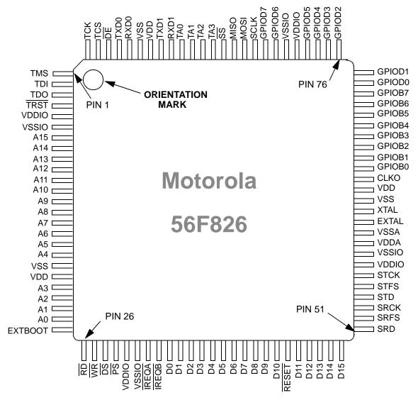
Figure 35. Top View, 56F826 100-pin LQFP Package
