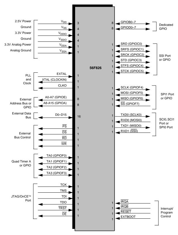
Figure 2. 56F826 Signals Identified by Functional Group<sup>1</sup>
