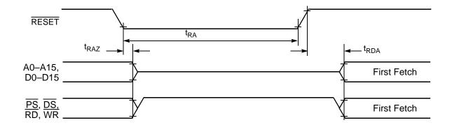
**Figure 16. Asynchronous Reset Timing**
