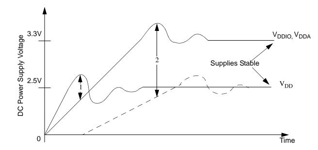
Notes: 1.  $V_{DD}$  rising before  $V_{DDIO}$ ,  $V_{DDA}$
