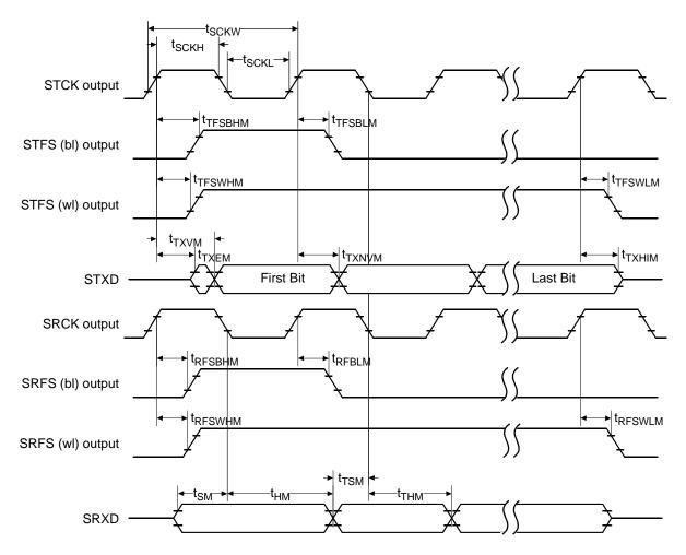
Figure 26. Master Mode Timing Diagram
