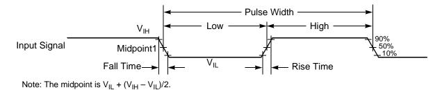
Figure 6. Input Signal Measurement References
