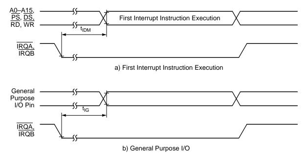
Figure 18. External Level-Sensitive Interrupt Timing
