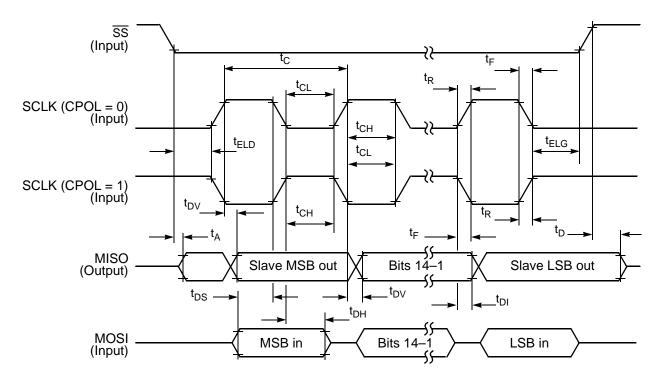
Figure 25. SPI Slave Timing (CPHA = 1)
