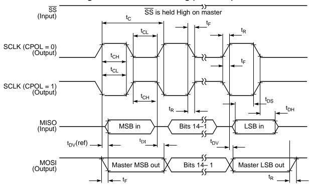
Figure 23. SPI Master Timing (CPHA = 1)
