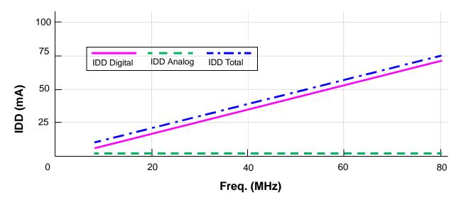
Figure 3. Maximum Run IDD vs. Frequency (see Note 6. in Table 7)
