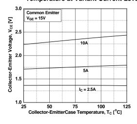
**Figure 2. Typical Output Characteristics**
