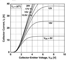
Figure 3. Typical Saturation Voltage Characteristics
