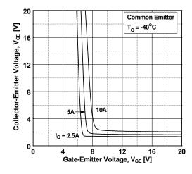
Figure 7. Saturation Voltage vs. V<sub>GE</sub>
