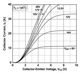
**Figure 4. Transfer Characteristics**
