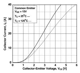
Figure 5. Saturation Voltage vs. Case
