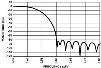
FIGURE 14. DIGITAL-TO-ANALOG PASSBAND FREQUENCY RESPONSE (FULL SCALE INPUTS, 0dB)
