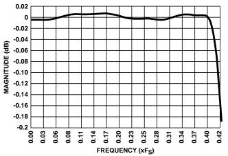
FIGURE 10. ANALOG-TO-DIGITAL FREQUENCY RESPONSE (FULL SCALE LINE INPUTS, 0dB)
