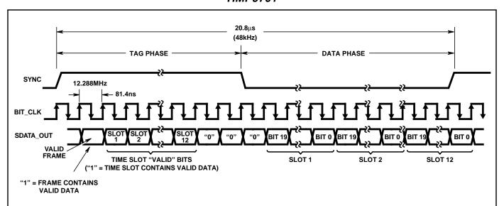
FIGURE 3. AC LINK AUDIO OUTPUT FRAME
