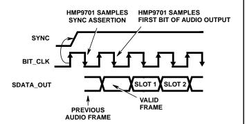
FIGURE 4. START OF AUDIO OUTPUT FRAME
