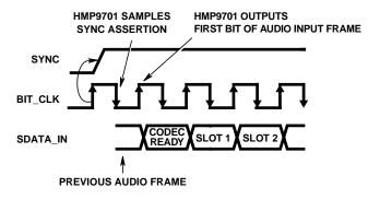
FIGURE 5. START OF AUDIO INPUT FRAME
