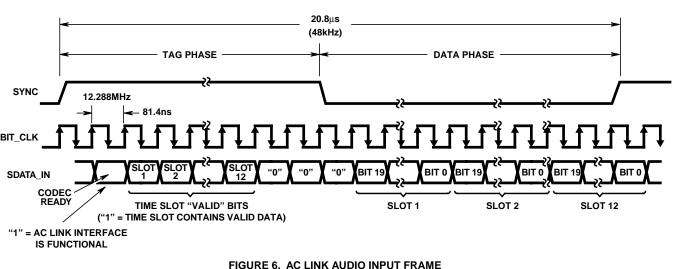
FIGURE 6. AC LINK AUDIO INPUT FRAME
