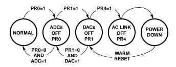
FIGURE 9. HMP9701 POWERDOWN/UP WITH ANALOG ALIVE
