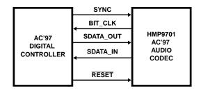
FIGURE 1. HMP9701 CONNECTION TO AC'97 CONTROLLER
