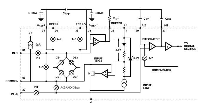
FIGURE 3. ANALOG SECTION OF ICL7106 AND ICL7107
