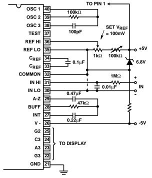
Since low TC zeners have breakdown voltages  $\sim$  6.8V, diode must be placed across the total supply (10V). As in the case of Figure 14, IN LO may be tied to either COMMON or GND.
