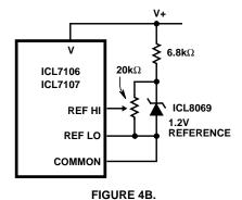
FIGURE 4. USING AN EXTERNAL REFERENCE
