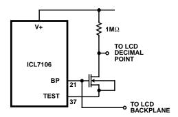
FIGURE 5. SIMPLE INVERTER FOR FIXED DECIMAL POINT
