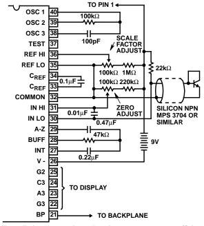
A silicon diode-connected transistor has a temperature coefficient of about -2mV/°C. Calibration is achieved by placing the sensing transistor in ice water and adjusting the zeroing potentiometer for a 000.0 reading. The sensor should then be placed in boiling water and the scale-factor potentiometer adjusted for a 100.0 reading.
