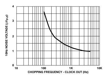
FIGURE 12. 10Hz NOISE VOLTAGE vs CHOPPING FREQUENCY
