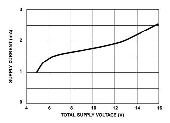
FIGURE 7. SUPPLY CURRENT vs SUPPLY VOLTAGE
