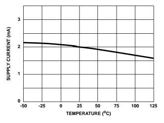
FIGURE 8. SUPPLY CURRENT vs AMBIENT TEMPERATURE
