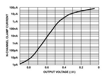
FIGURE 20. N-CHANNEL CLAMP CURRENT vs OUTPUT VOLTAGE
