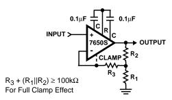
NOTE:  $R_1||R_2$  indicates the parallel combination of  $R_1$  and  $R_2$ . FIGURE 2. NON INVERTING AMPLIFIER WITH OPTIONAL CLAMP
