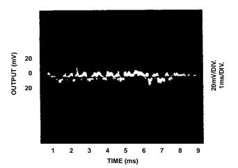
FIGURE 15. OUTPUT WITH ZERO INPUT; GAIN = 1000; BALANCED SOURCE IMPEDANCE =  $10k\Omega$
