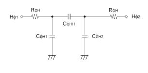
Vertical transfer clock equivalent circuit
