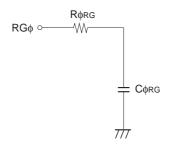
Reset gate clock equivalent circuit
