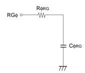
Reset gate clock equivalent circuit
