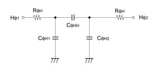
Vertical transfer clock equivalent circuit
