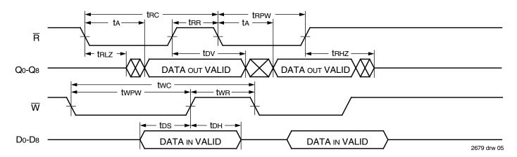
Figure 3. Asynchronous Write and Read Operation
