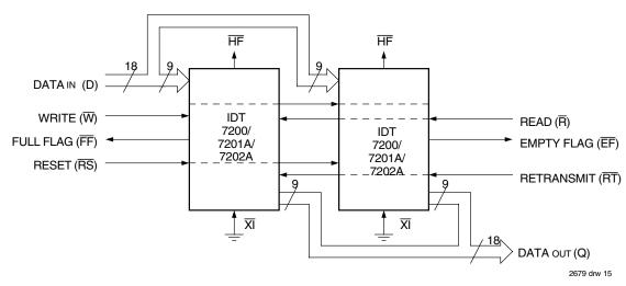
Figure 13. Block Diagram of 256 x 18, 512 x 18, 1,024 x 18 FIFO Memory Used in Width Expansion Mode
