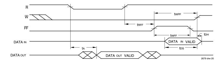
Figure 18. Write Data Flow-Through Mode
