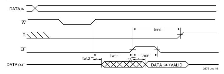
Figure 17. Read Data Flow-Through Mode
