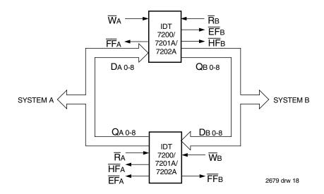
Figure 16. Bidirectional FIFO Mode
