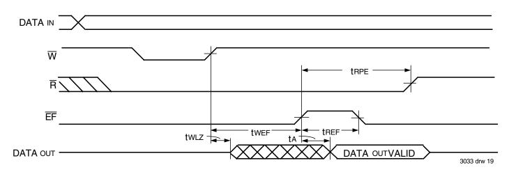
Figure 17. Read Data Flow-Through Mode
