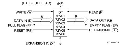
Figure 12. Block Diagram of Single 512 x 9, 1,024 x 9, 2,048 x 9, 4,096 x 9, 8,192 x 9 and 16,384 x 9 FIFO
