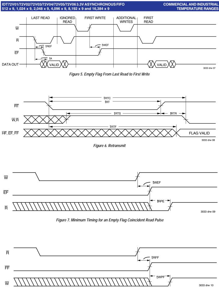
Figure 8. Minimum Timing for a Full Flag Coincident Write Pulse
