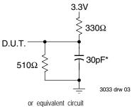
Figure 1. Output Load
