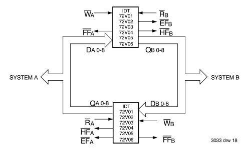
Figure 16. Bidirectional FIFO Mode
