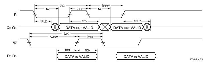
Figure 3. Asynchronous Write and Read Operation
