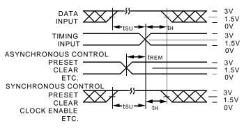
Set-up, Hold, and Release Times
