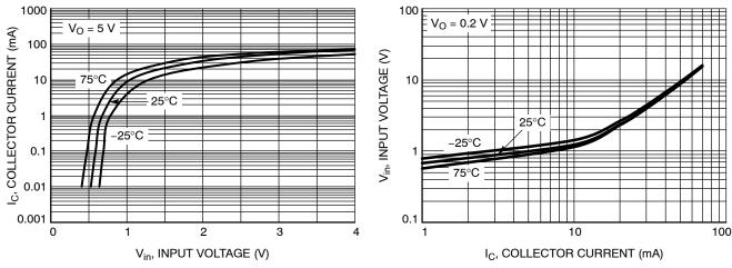
Figure 3. Output Current vs. Input Voltage
