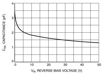
Figure 5. Output Capacitance
