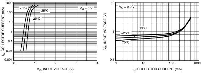
Figure 8. Output Current vs. Input Voltage
