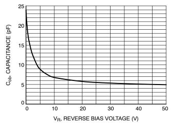
Figure 10. Output Capacitance
