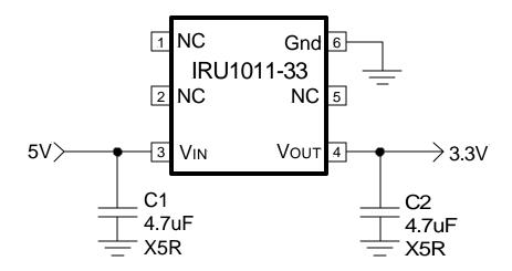
Figure 1 - Typical application of IRU1011-33.
