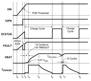
FIGURE 2. TIMING DIAGRAM AFTER AN ADAPTER IS ATTACHED TO THE CHARGER INPUT.
