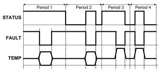
FIGURE 5. EFFECTS OF THE TEMP PIN.
