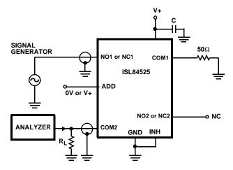
FIGURE 6. CROSSTALK TEST CIRCUIT
