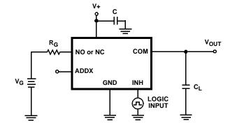
FIGURE 2A. MEASUREMENT POINTS
