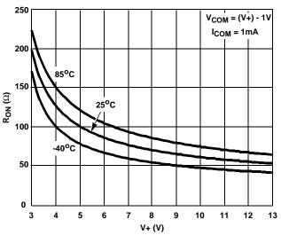
FIGURE 9. ON RESISTANCE vs SUPPLY VOLTAGE
