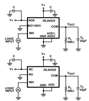
Repeat test for other switches. C<sub>L</sub> includes fixture and stray capacitance.
