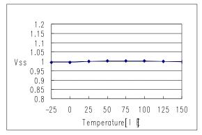
Figure 13. Soft Start Voltage
