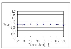
Figure 12. Over Voltage Protection
