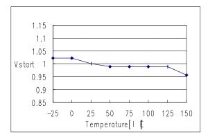
Figure 6. Start Threshold Voltage
