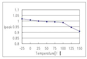
Figure 4. Max. Inductor Current
