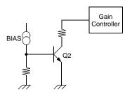
When the chip temperature rises up to about 175°C, the Q2 turns on so that the output driver will be shutdown. When the chip temperature falls off to about 150°C, then the Q2 turns off so that the driver is to operate normally. Thus, TSD has the temperature hysteresis of about 25°C.
