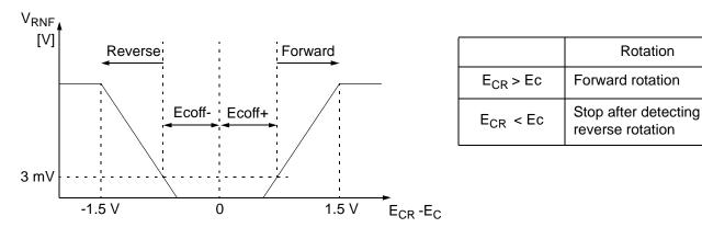
The input range of E<sub>CR.</sub> E<sub>C</sub> is 0.2 V ~ 4 V
