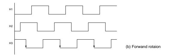
Therefore, the output of the rotational direction detector is Low, when the spindle rotates forward, while HIGH as in the case of the reverse rotation.
