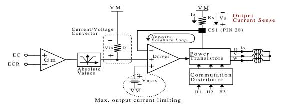
0.255 which is made from GM times R1 is fixed value within IC.
