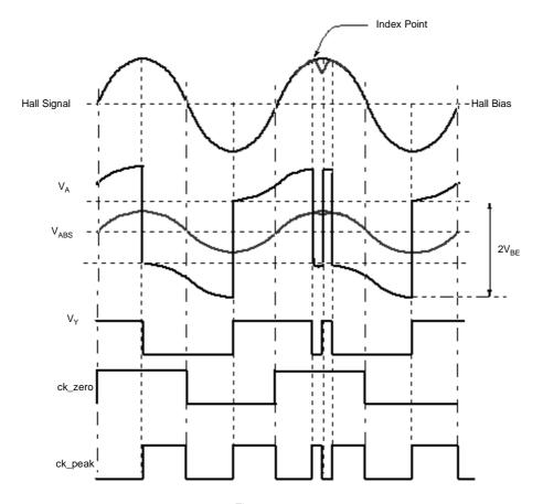
V<sub>ABS</sub> in the figure4-1 is a signal from twice amplified hall signal and hall bias at 2.5volt as standard voltage as you see in the figure 4-2.
