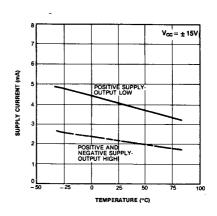
Figure 8. Supply Current vs Temperature
