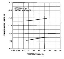
Figure 5. Common Mode Limits vs Temperature
