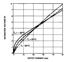
**Figure 11. Current Saturation Voltage**
