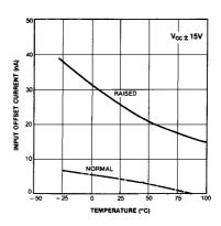
Figure 2. Input Offset Current Vs Temperature
