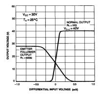
Figure 6. Output Voltage vs Differential input voltage
