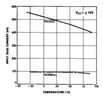
Figure 1. Input Bias Current Vs Temperature
