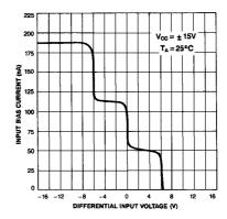
Figure 4. Input Bias Current vs Dfferential input voltage
