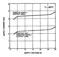
Figure 10. Supply Current vs Supply Voltage
