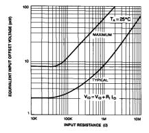
Figure 3. Offset Voltage vs Input Resistance
