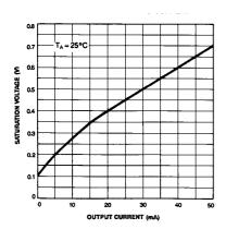
Figure 7. Saturation voltage vs Current
