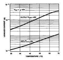
Figure 9. Leakage Current vs Temperature
