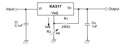
$V_0 = 1.25V (1+R_2/R_1)+I_{adj}R_2$
