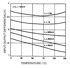
Figure 3. Dropout Voltage
