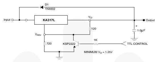
Figure 2. 5V Electronic Shutdown Regulator
