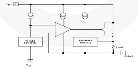
Figure 1. Block Diagram
