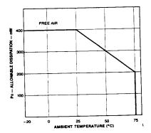
Figure 7. Allowable Dissipation vs.
