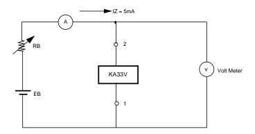
Figure 1. Measuring Circuit for Stabilized Voltage Vz
