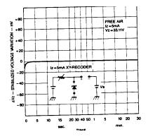
Figure 10. Stabilized Voliage Variation vs. Time
