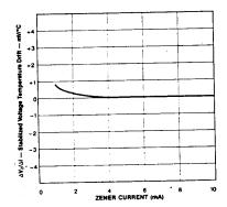
Figure 9. Stabilized Voltage Temperature Drift vs. Zener Current
