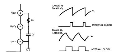
Figure 5. Oscillator Waveforms and Maximum Duty Cycle
