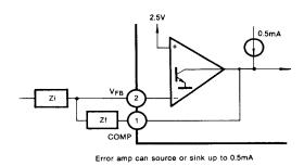
Figure 3. Error Amp Configuration
