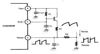
Figure 9. Slope Compensation
