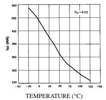
Figure 11. Temperature Drift (Ist)
