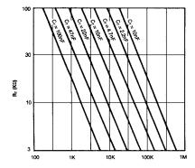
Figure 7. Timing Resistance vs Frequency
