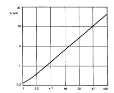
Figure 6. Oscillator Dead Time & Frequency
