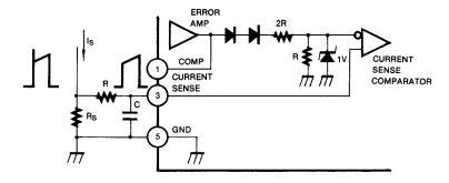
Figure 4. Current Sense Circuit
