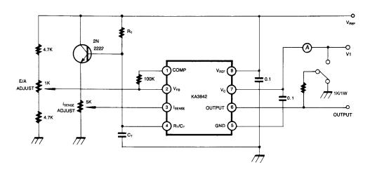
Figure 1. Open Loop Test Circuit
