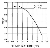
Figure 10. Temperature Drift (Vref)
