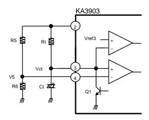
If the UP/DOWN switch is pushed less than a set time(Ts), TR(Q1) will be turned off and capacitor(Ct) is charged exponentially until Vct equals to V5. At that time TR(Q1) is turned on and stops the operation.
