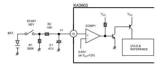
In the state of the START-KEY turned OFF, all the blocks in the KA3903 are kept to be OFF because the power is not supplied into UVLO block.
