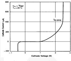
Figure 6. Cathode Current vs. Cathode Voltage
