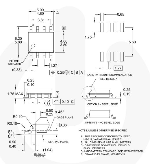
Figure 19. 8-Lead, SOIC, JEDEC MS 0-12, 0.150 inch Narrow Body
