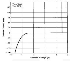
Figure 5. Cathode Current vs. Cathode Voltage
