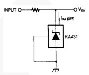
Figure 4. Test Circuit for I<sub>KA(OFF)</sub>
