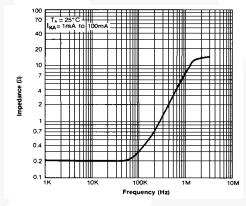
Figure 8. Dynamic Impedance Frequency
