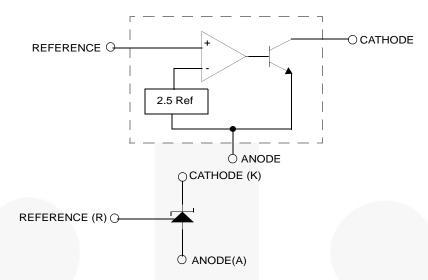
Figure 1. Block Diagram
