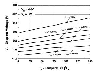
Figure 1. Dropout Voltage
