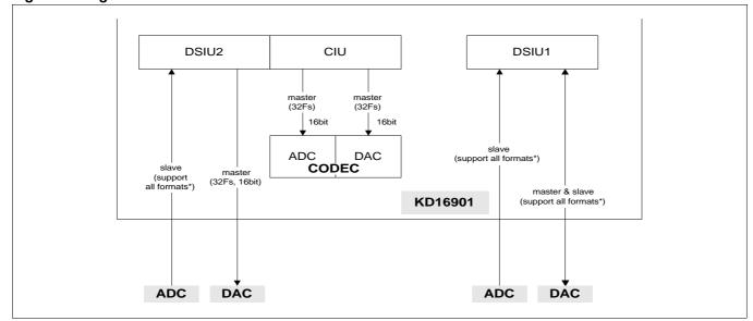
Figure 3. Digital Audio Interface Formats of the KD16901
