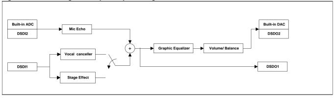
Figure 27. Block Diagram of Input/Output Configuration 5
