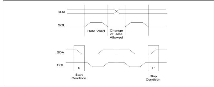
Figure 8. Data Validity and Start/Stop Condition in PC Bus
