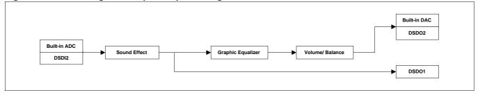
This configuration is exactly same as Configuration 1 except for input source. For this configuration, one should set Mixing and Bypass On-Chip Function to be turned off while the built-in ADC or DSDI2 is enabled. To obtain Configuration 3, one can send host commands from microcontroller in the order of the commands listed in Table 15.
