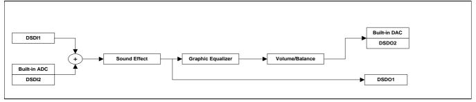
For this configuration, one should set Mixing to be turned on and Bypass On-Chip Function to be turned off. Input signals from different sources can be mixed with controllable gains. After mixed, the flow is identical to Configuration 1 and 3. To obtain Configuration 4, one can send host commands from microcontroller in the order of the commands listed in Table 16.
